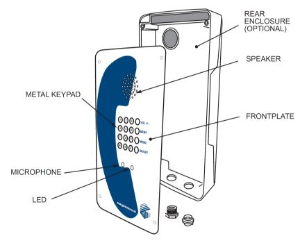
This manual describes Sentinel hands-free telephone products. These units offer high degrees of resistance to weather and abuse, having only a microphone, speaker and a rugged metal keypad mounted on a flat, metal faceplate, in place of a traditional handset. Main features include:
