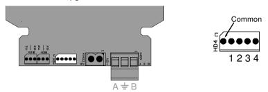
The inputs are provided on HD4 as shown, and are also labelled on the circuit board. Control inputs are for connection to voltage free contacts only. Internal pull-up resistor source current =  $33\mu$ A. These inputs form part of a TNV3 circuit and precautions must be taken to prevent hazardous voltages being applied to these circuits.
